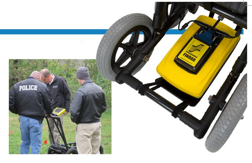
FINDAR is a GPR system specifically designed to meet the needs of law enforcement and military professionals. Designed, engineered and optimized specifically for evidence collection in current investigations and cold cases, FINDAR provides quick and accurate data acquisition enabling law enforcement professionals to locate buried evidence.
